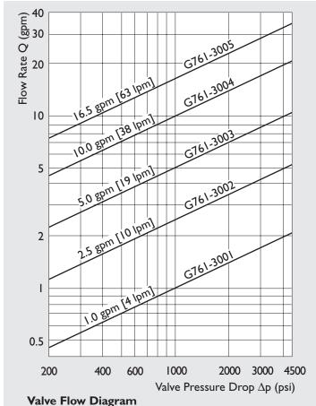
Valve flow for maximum valve opening (100% command signal) as a function of the valve pressure drop.
